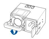
2. Hold the PSU lever and press the PSU latch inwards, then carefully pull the PSU out of the system chassis.
