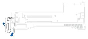
Install the expansion card, then push the slot cover lock inwards to secure the expansion card.
