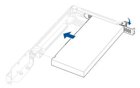
4. Install the expansion card bracket and tighten the thumbscrew.
