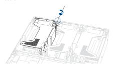
2. Press the latch inwards, then lift and remove the expansion card bracket.
