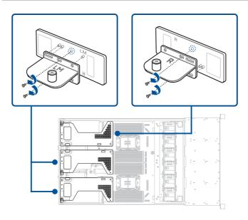
3. Install the airflow blocker, then tighten the thumbscrew.
