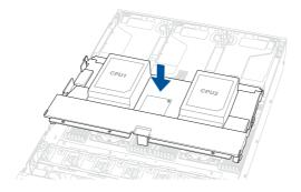
2. Install the metal bracket, then return the latches to the locked position.
