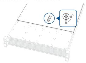
2. Press the spring lock to release the latch, then pull the latch upwards to disengage the chassis cover from the chassis.
