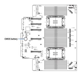
2. Place the replacement CMOS battery into the battery compartment.
