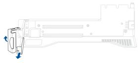
Install the GPU card, then push the slot cover lock inwards to secure the expansion card.
