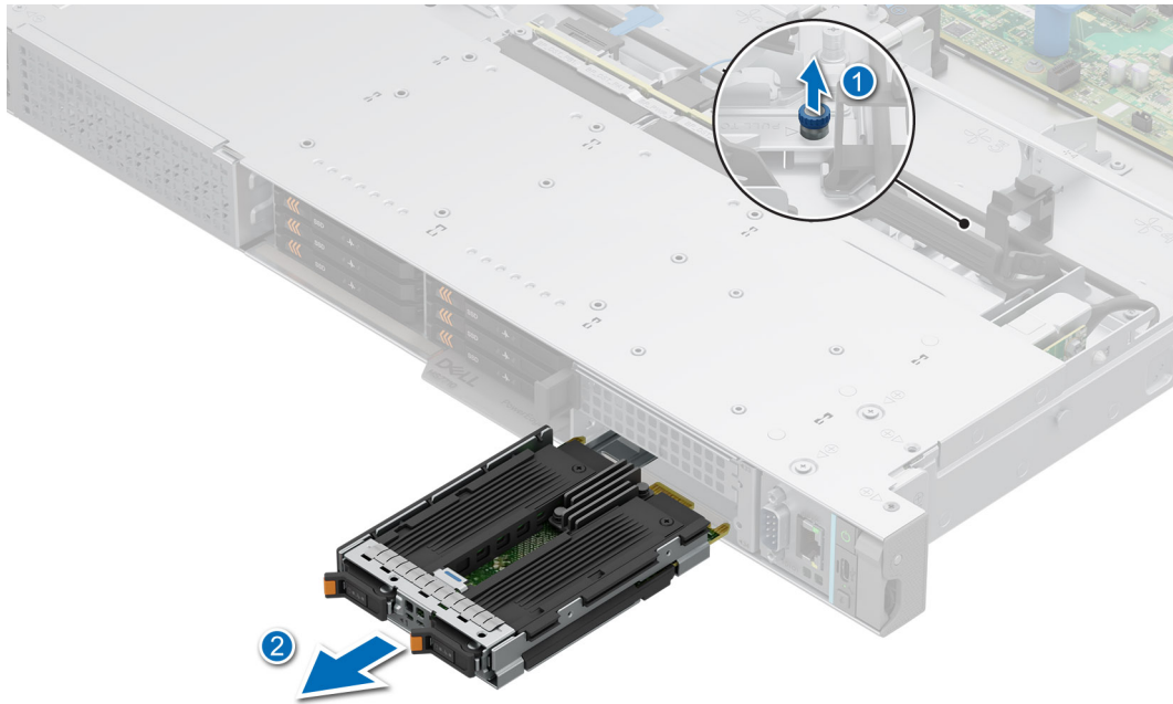
Figure 195. Removing a BOSS-N1 DC-MHS module tray from the system
