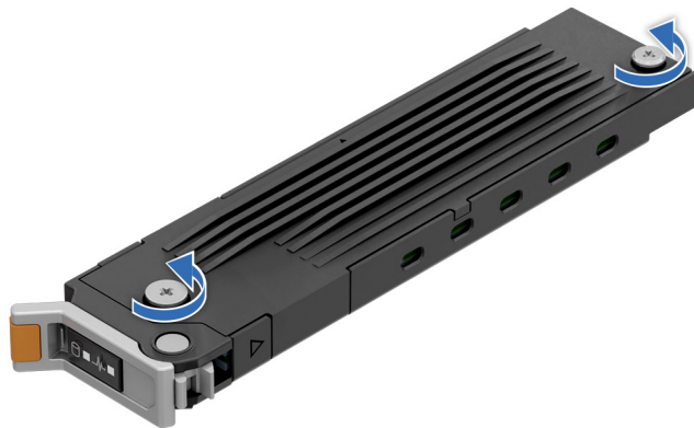
Figure 171. Loosen the top cover captive screws
