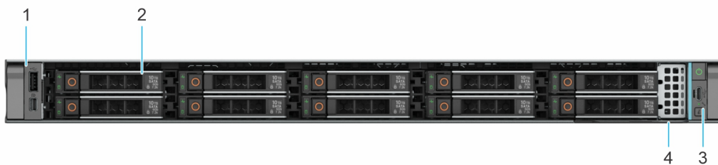
Figure 2. Front view of 10 x 2.5-inch drive system
