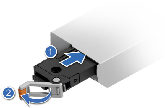
Figure 182. Installing the BOSS-N1 DC-MHS card carrier
