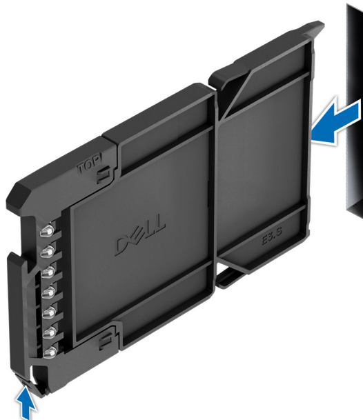
Figure 66. Removing an EDSFF E3.S drive blank
