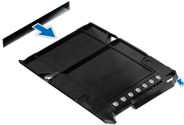
Figure 38. Removing an EDSFF E3.S Gen5 NVMe drive blank
