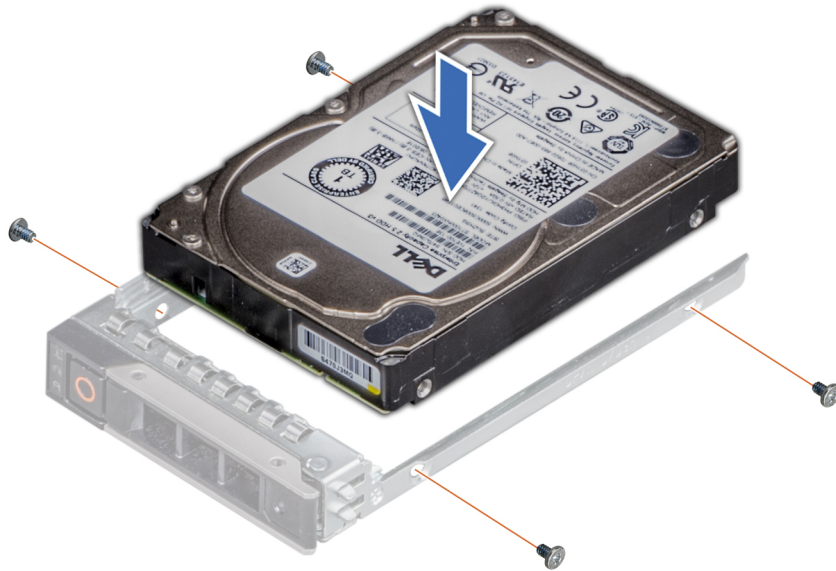
Figure 46. Installing a SSD drive into the drive carrier
