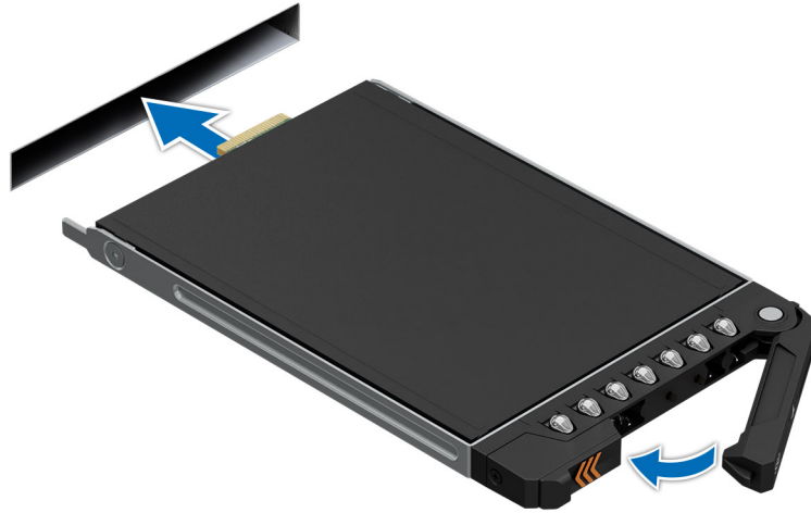
Figure 43. Installing an EDSFF E3.S Gen5 NVMe drive carrier
