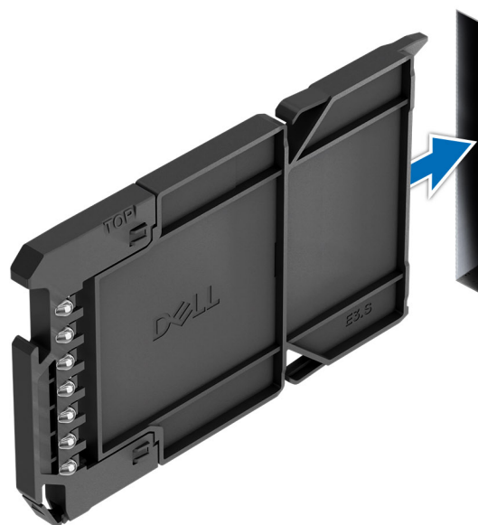
Figure 50. Installing an EDSFF E3.S drive blank
