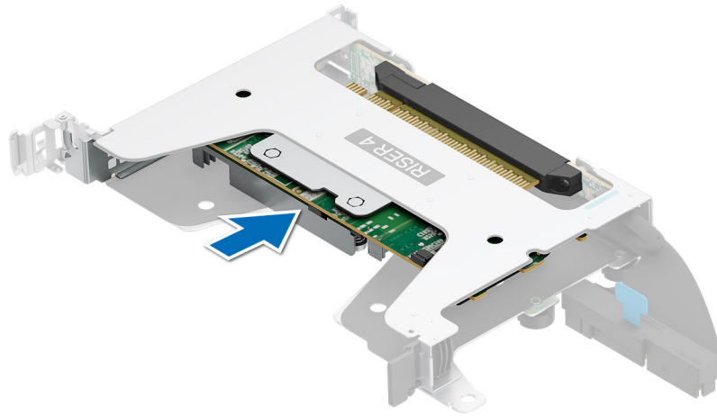
Figure 157. Installing an expansion card into the riser 4b
