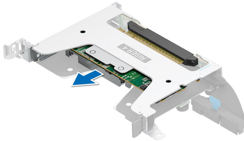
Figure 152. Removing low-profile expansion card from the riser 4b
