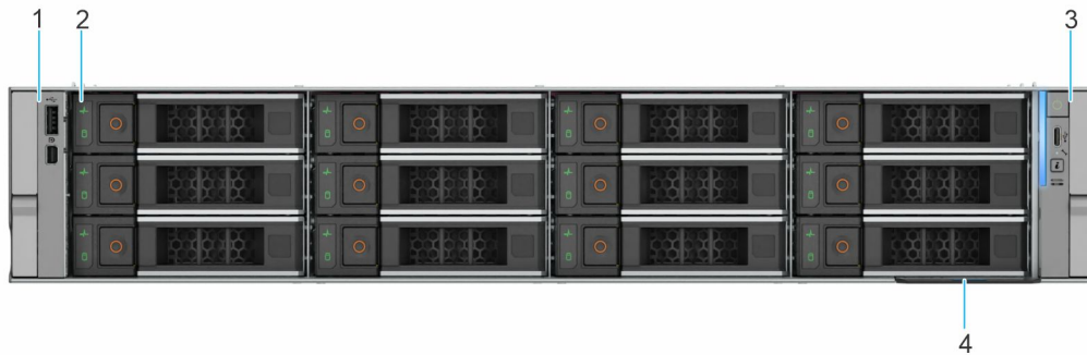
Figure 3. Front view of the 12 x 3.5-inch SATA/SAS
