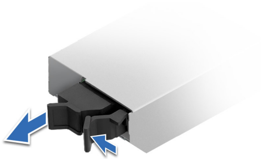
Figure 182. Removing the BOSS-N1 card carrier blank
