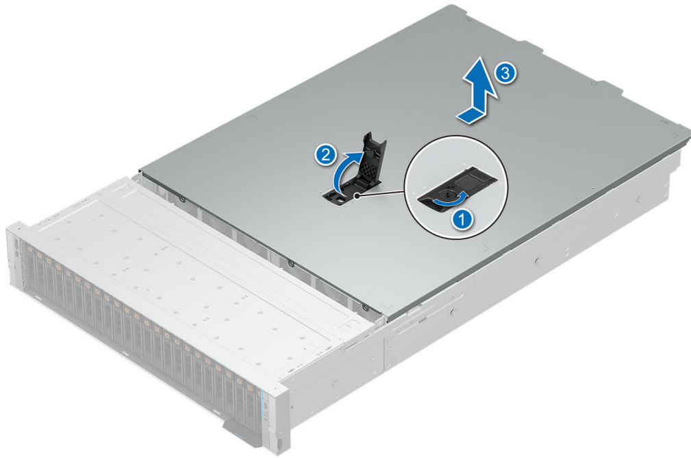
Figure 33. Removing the system cover
