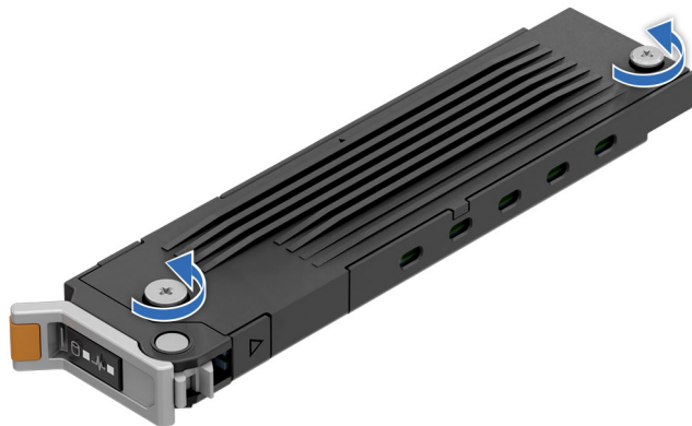
Figure 175. Loosen the top cover captive screws
