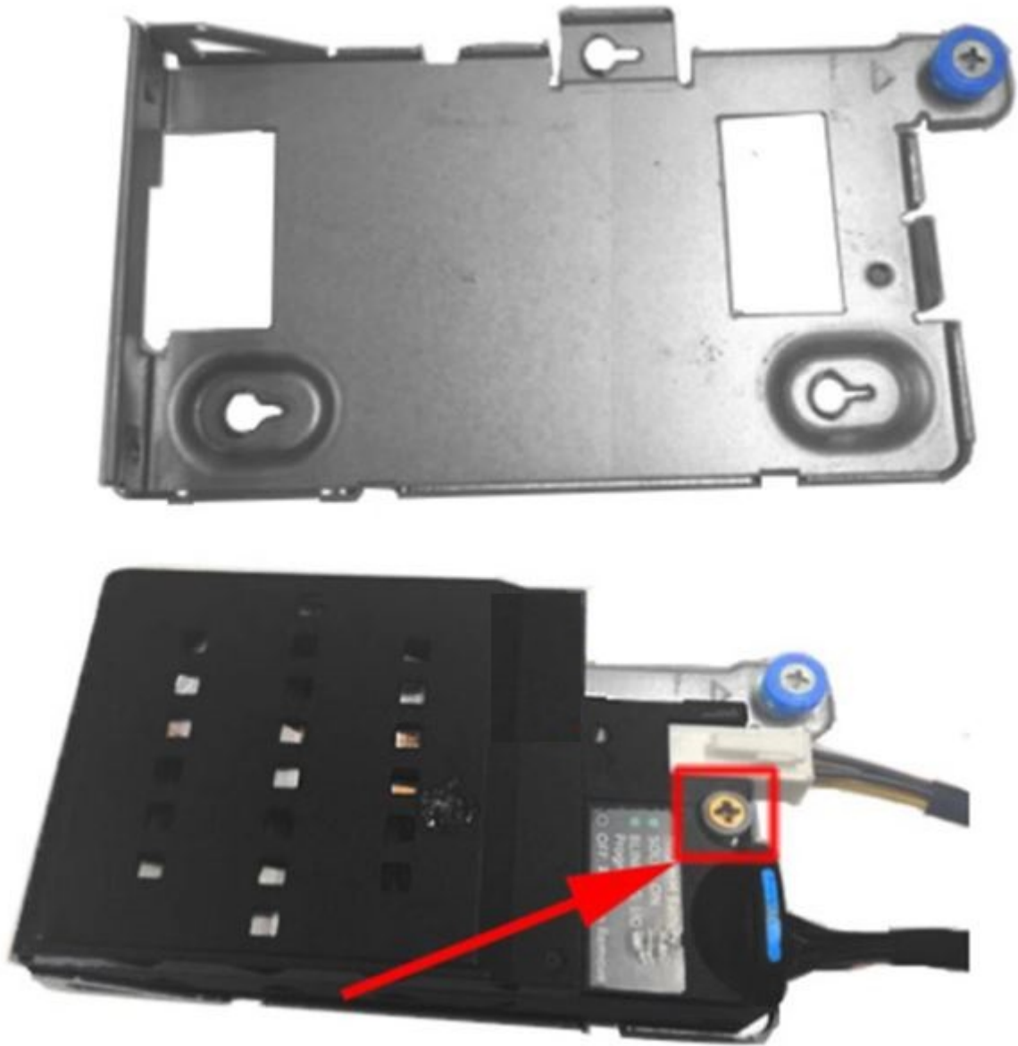
Figure 151. Installing battery on the battery tray
