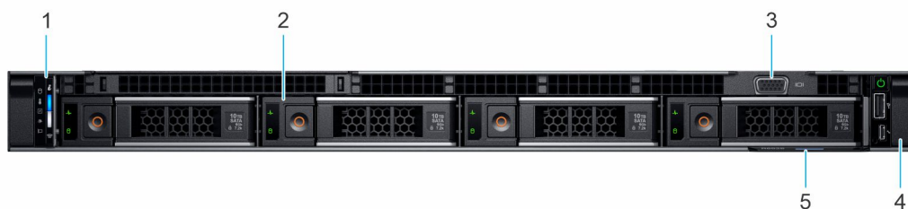
Figure 1. Front view of 4 x 3.5-inch SAS/SATA drive system
