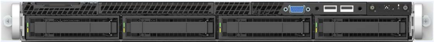
Figure 11. 3.5" x 4 front drive bay configuration – R1304WFxxxx
