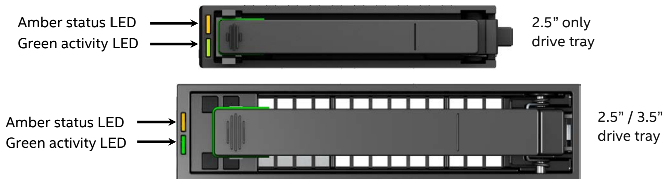
Figure 33. Drive tray LED identification
