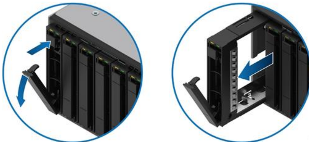
Figure 44. Drive carrier removal
