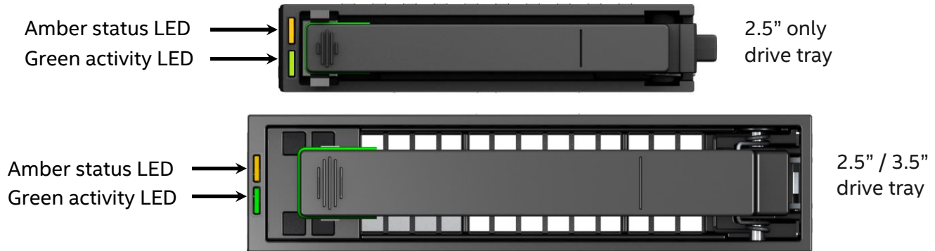
Figure 46. Drive tray LED identification
