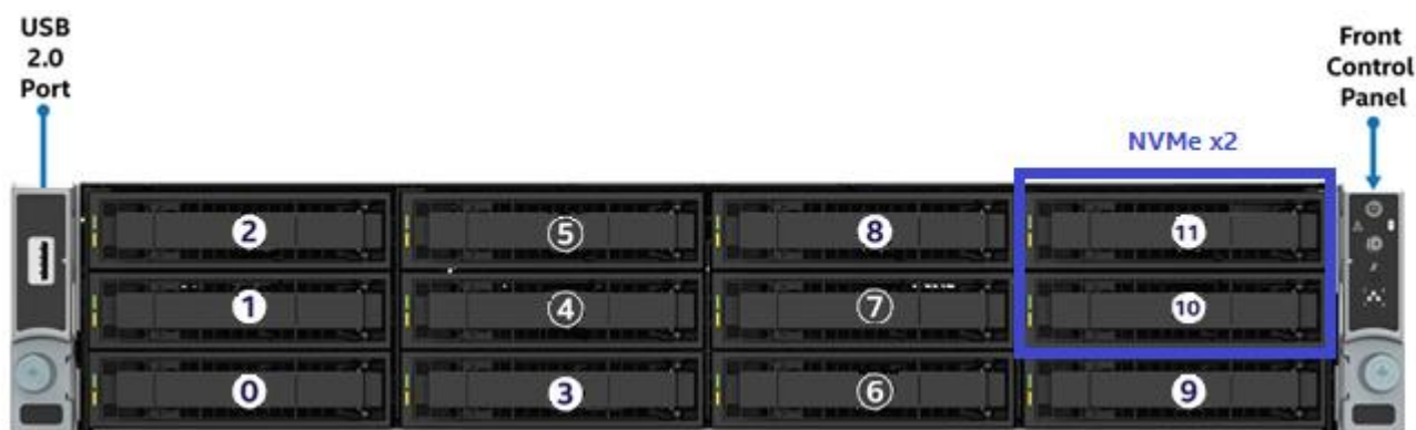
Figure 43. 3.5" drive bay, 12 drive configuration
