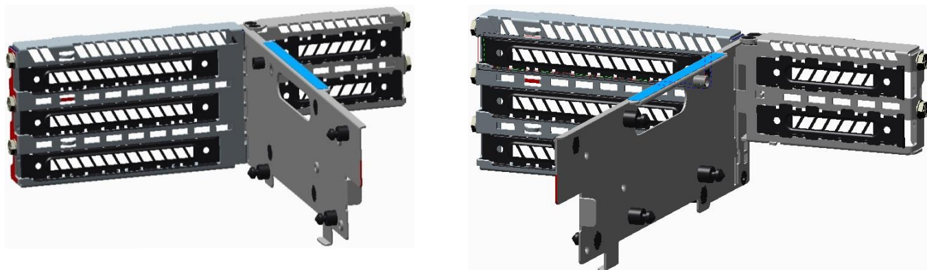
Figure 82. Left and right views of riser card #2 and #3 bracket
