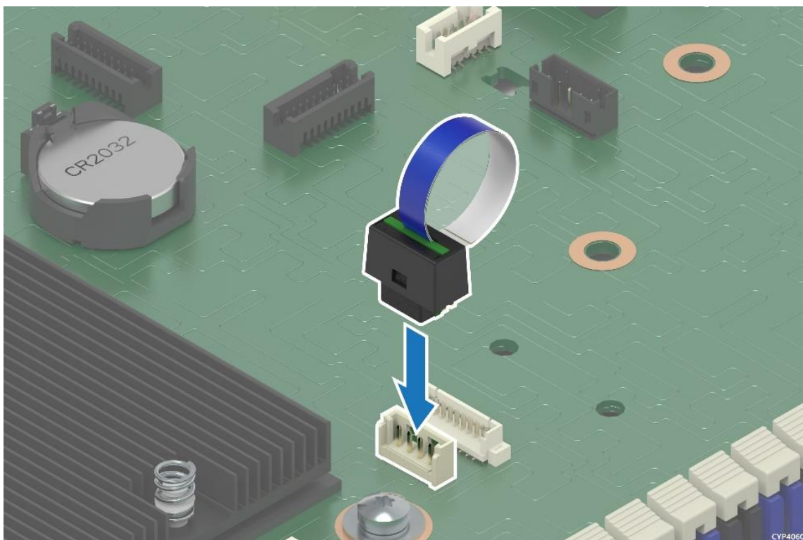
Figure 81. Intel® VROC Key Insertion
