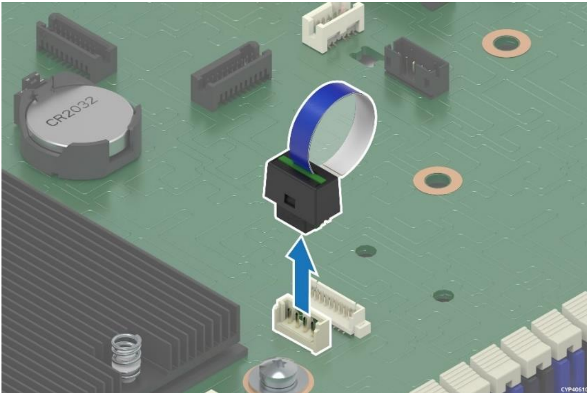
Figure 82. Intel® VROC Key Removal
