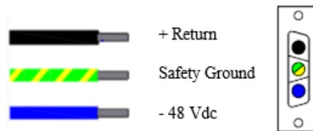
Figure 2-5. DC Input Power Cable Connector
