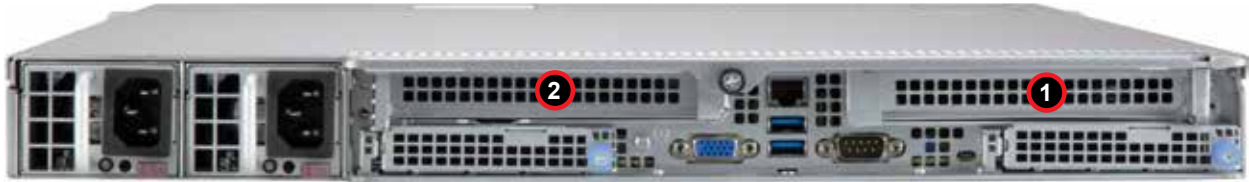
Figure 3-24. Expansion Card Slots in the Chassis
