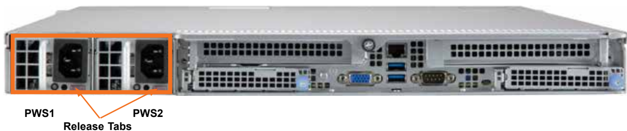
Figure 3-21. Replacing the Power Supply
