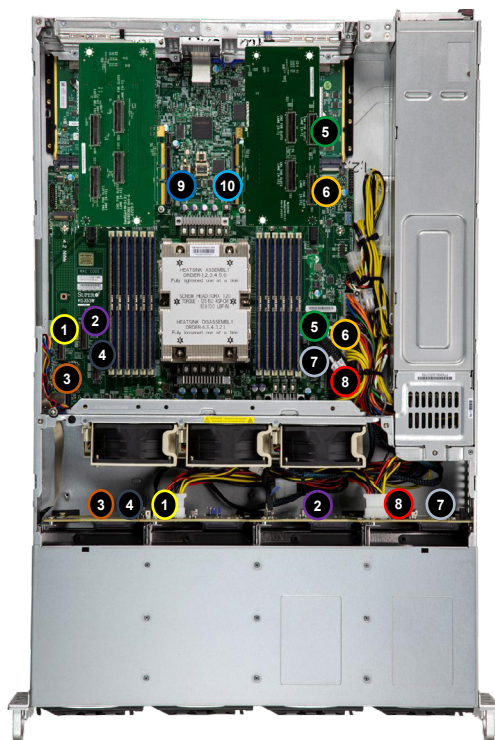
Figure 3-22. Cable Routing Diagram (12 NVMe + 2x PCIe x16)
