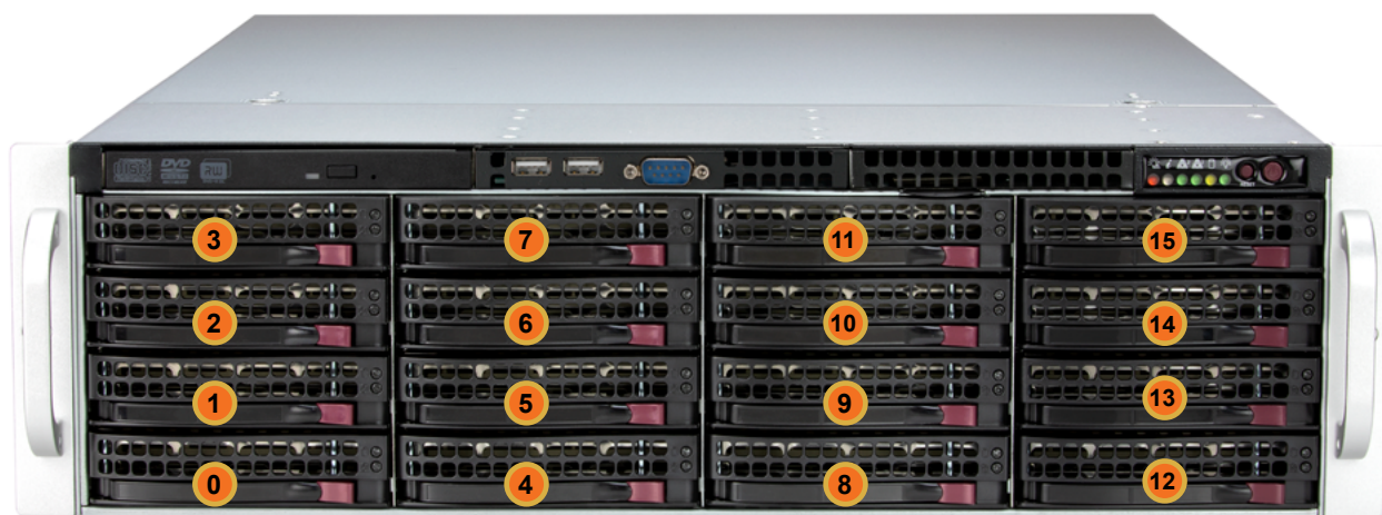
Figure 3-4. Logical HDD Bay Locations
